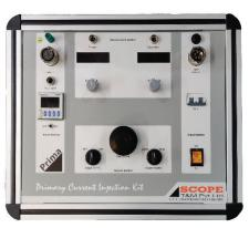
Prima consists of separate Control Unit and light weight Loading Unit which can be taken very near to the DUT terminals, reducing the requirement of the higher open circuit voltage & burden. Further, due to this arrangement, length of the output current leads got reduced and the overall weight of the kit got reduced substantially.
