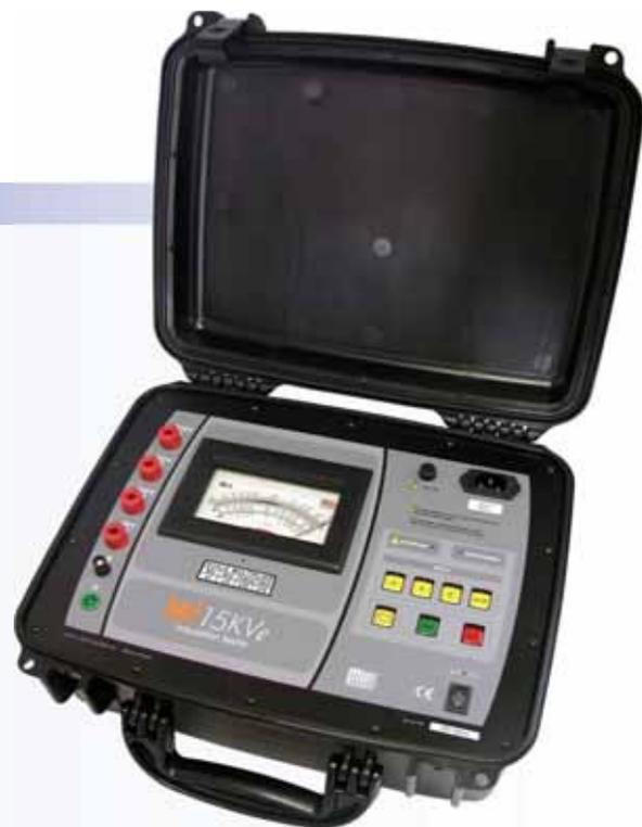
The MI-15KV<sub>e</sub> High-Voltage Megohmmeter is a truly portable device that allows the measurement of insulation resistances using test voltages up to 15kV. It employs a state-of-the-art technology for the safe measurements of insulation resistances up to 3.000.000M $\Omega$  with four test voltages: 1kV - 5kV - 10kV and 15kV. Readings are performed through an easy-to-read analogue indicator, having a broad scale.
