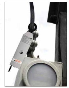
blocks. Resistive leakage current is in phase with the applied voltage, so it generates power loss in the form of heat. It may lead to cascading effect & accelerated failure of arresters.
