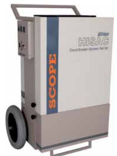
HISAC Ultima with 6 Channel DCRM mounted on Trolley
